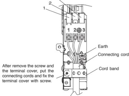
After remove the screw and the terminal cover, put the connecting cords and fix the terminal cover with screw.
