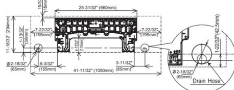
Screw the hanger at the positions possibly near the upper and lower hooks where the indoor unit is hung. Use 4 or more screws to fix the hanger.
